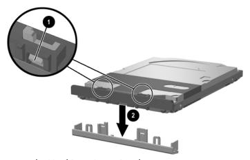
Removing the Hard Drive Lower Bezel
